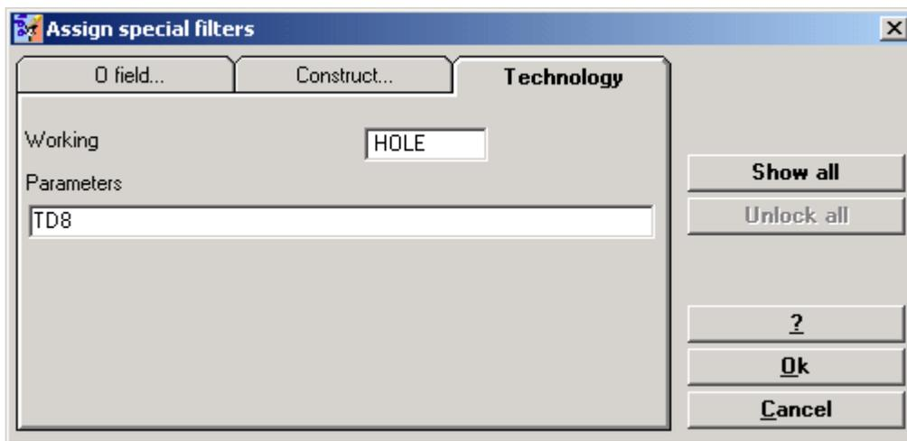
According to the data set in the example window the only workings with "HOLE" ASCII code and TD parameter value set to 8 are displayed.
