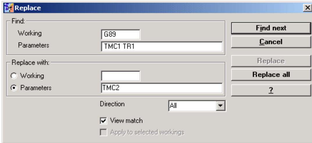
The setting parameters shown in this second Figure need a replacement of operating code. The "G89" workings are the only ones to be replaced with "G88" workings.
