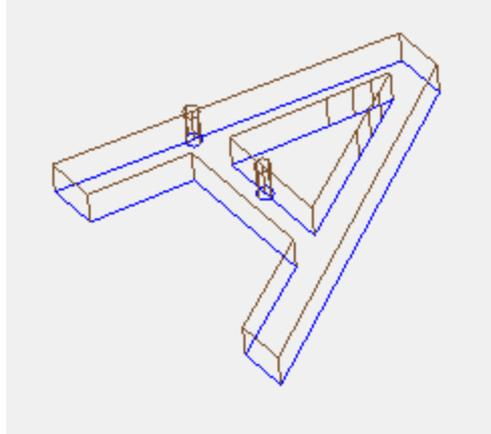
The drawing shows a 3D representation example of profiles, with the overall dimensions view enabled: each profile segment underlines the tool overall dimension in the piece. The default is disabled.
