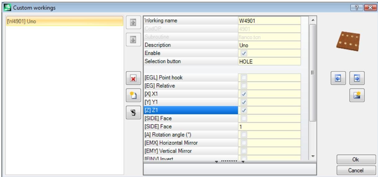
To create a complex working, select the button
