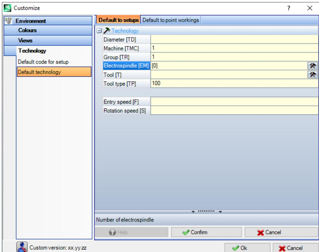
The tab is shown only if the working used to assign the default technology is in the workings database. The choice of the technology is not different for face and it is about the technological assignments of a general point or setup working.
