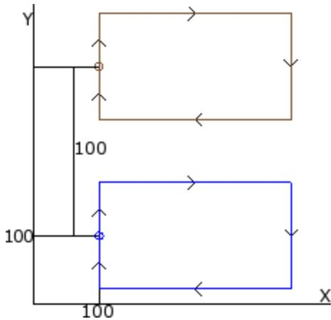
The figure corresponds to two applications of the subroutine in the example (making a rectangle):
