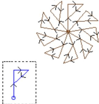
The section highlighted in figure corresponds to the single element as programmed in the subroutine. All repetitions are applied to the base application point and rotated to complete the round angle.
