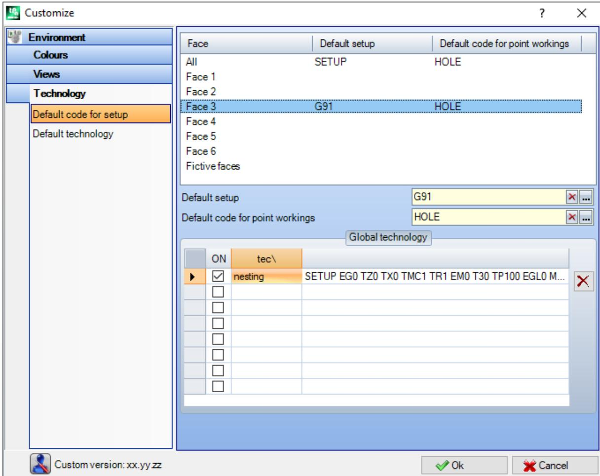
In the grid the technologies used for point and setup workings are assigned when a default assignment is required.
