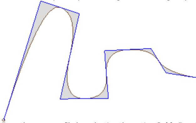
From the same profile by selecting the option **Cubic B-spline** we get the curve:
