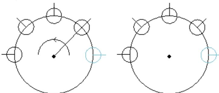
Repetition of the working marked with a bold line for **5** elements, angle to fill up: **180°**, counterclockwise rotation. The left figure shows the series whose **Rotate item in the series** field is not selected. The right figure shows the series whose **Rotate item in the series** field is selected.
