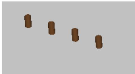
The drawing shows a 3D impersonation example of point workings (or isolated setups), that have an overall dimensions view: for each working is represented a little cylinder that is as high as the programmed depth. The little cylinder fill is determined by the selection **Show extent of points and setups with full segment**. The default setting is disabled.
