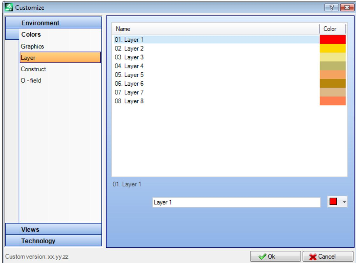
The table dimension is based on several rows (8 in the picture) equal to the maximum number that can be assigned to levels and, in any case, for a maximum number of 16. Property values bigger than 16 apply the colour that is here assigned for the 16 value.
