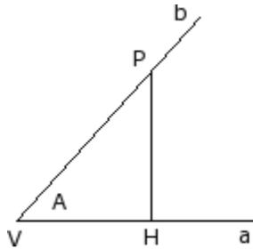
The user should remember that an angle is defined as positive when it rotates in counterclockwise direction. Let us consider an angle **(A)**: (in radians) of vertex **V** and sides **a** and **b**. Let us take on the half-line **b** any point **P** distinct from the vertex **V**. Let us project it on the half-line **a**: be **H** the point of the perpendicular described by **P** on **a**.
