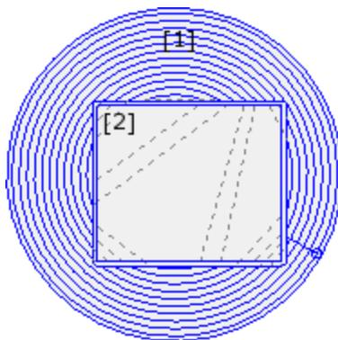
In the figure: the emptying process of a circle (1) with rectangular island (2).
