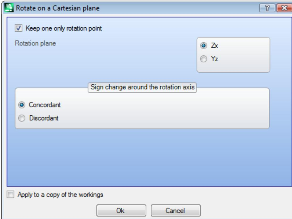
This tool rotates the profiles(s) of 90° around one of the two coordinated axes of the face plane. The possible options are:
