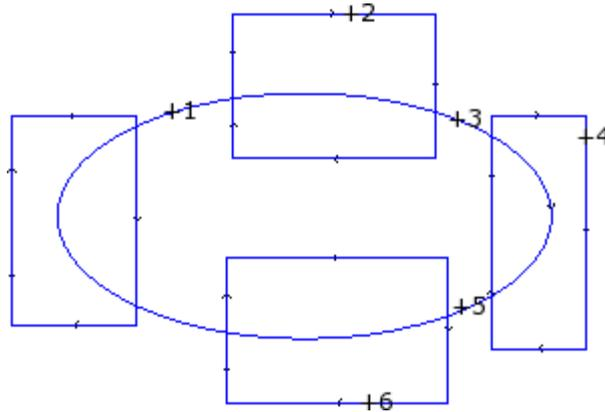
The Figure shows a program made of intersecting profiles. The 6 crosses identify the indicated parts for the construction of a new profile. Crosses are numbered and indicate the order by which the selected parts are added to the new profile:
