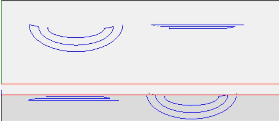
By selecting the option *Apply to a copy of the workings* the tool is applied to a copy of the workings and it does not modify the original lines.
