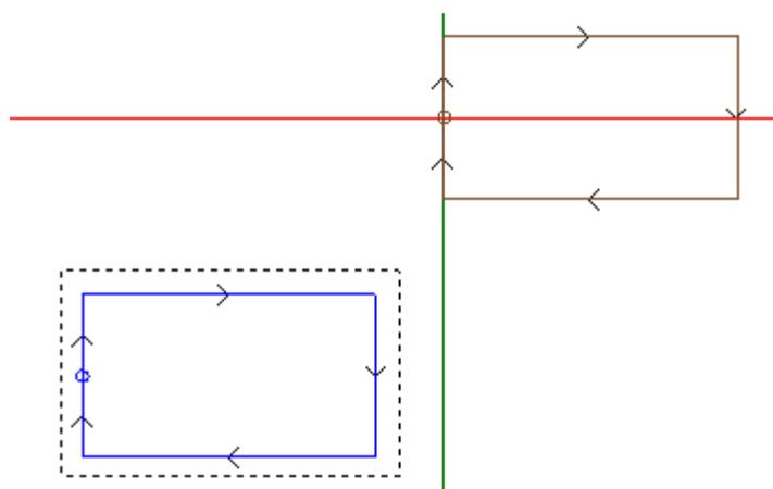
The rectangle selected in figure represents the subroutine development (a rectangle crossed clockwise, with start point located in the middle of the left vertical side).
