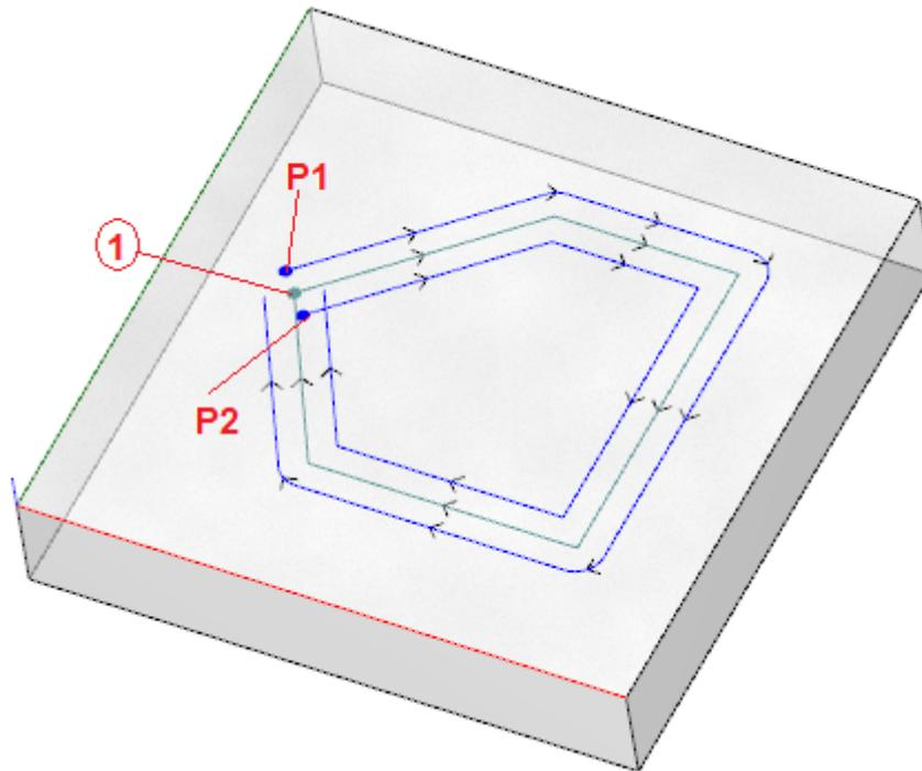
The central profile corresponds to the programmed profile: the setup is indicated as a point (1); (P1) shows the setup of the profile taken through left Compensation; (P2) shows the setup of the profile taken through right Compensation.
